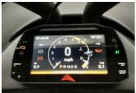
5. The LCD display is activated, now the trike is ready to start the engine.
