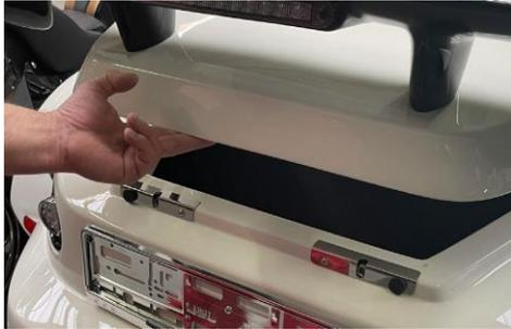
2. now you can open the trunk lid on the back of the trike upwards.
